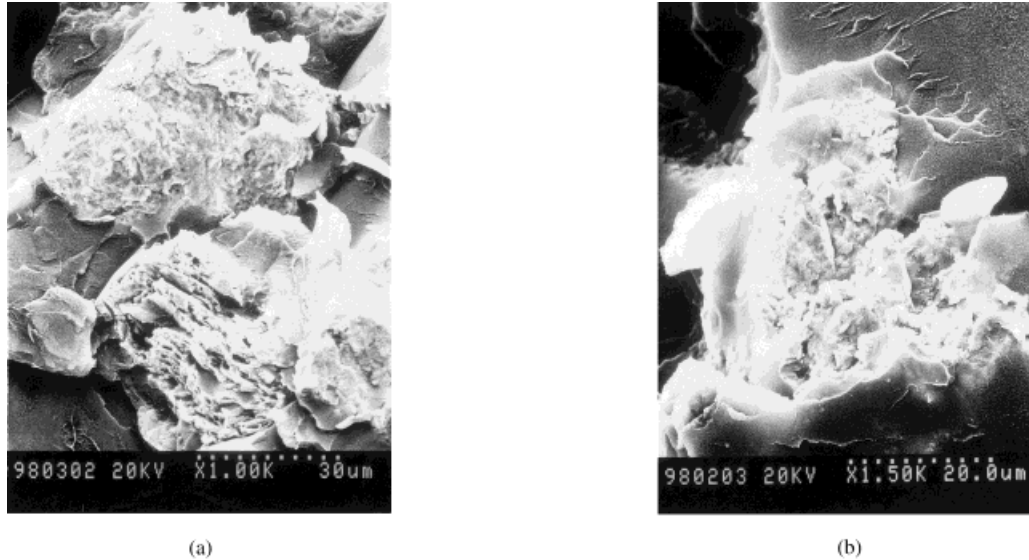
Figure 7 Scanning electron micrographs for the fracture surfaces of composites (a) as-prepared and (b) quenched in ice/water mixture from 240°C.
